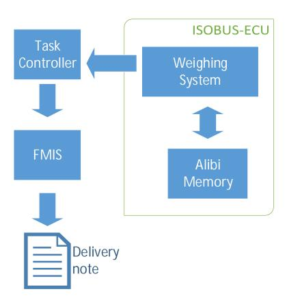
Alibi memory is fix connected to ISOBUS weighing system by an internal connection. Review might be possible through a VT mask or similar method.
